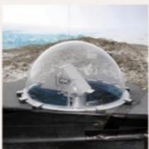
Upper Atmosphere Wind Observations: Fabry-Perot Interferometer Network
